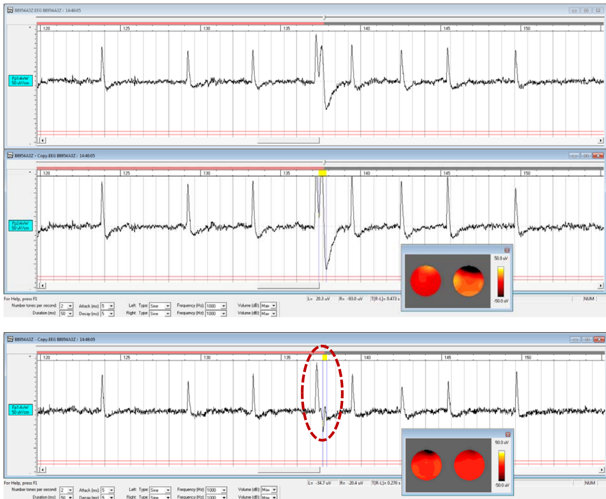
Fig 3. Eyeblinks visible in the EEG: (a) in the raw EEG, comparing traces for electrodes Fp1 and Fp2; (b) as 'inverted' ICA artefacts (showing apparent blink as another type of artefact)
